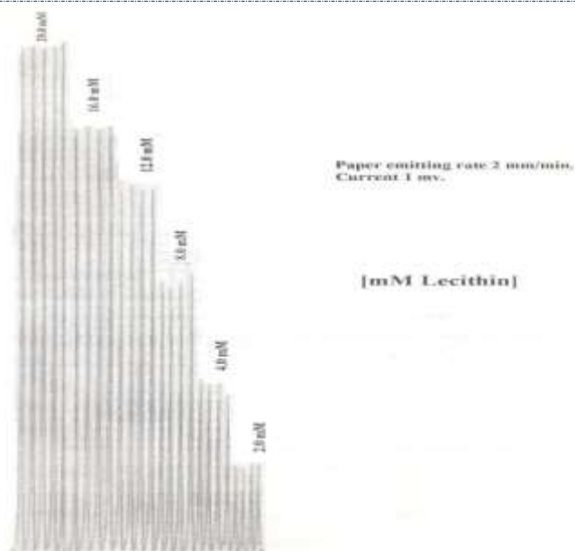
Fig. 7: Recorder output for varying concentration of lecithin, catalyzed by immobilized PLD and Choline Oxidase.
